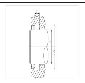
Rod seals are designed to seal the pressurized hydraulic fluid against the atmosphere, preventing leakage and pollution of the environment.
