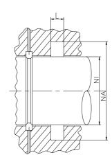
Rotary seals are designed to seal the pressurized hydraulic fluid against the atmosphere, preventing leakage and pollution of the environment or to transfer liquids and/or gases from a stationary part into or out of rotating machinery.
