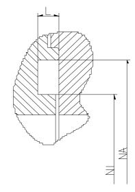
The flange seal FL06 is a symetric, spring energized seal for axial sealing applications. The geometry is leant against profile PRS19.
