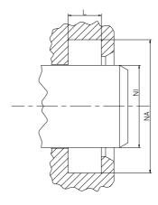
Wipers are designed to keep dust, dirt, sand and others off the rod and the sealing and guiding elements, avoiding abrasive damage caused by external contamination.
